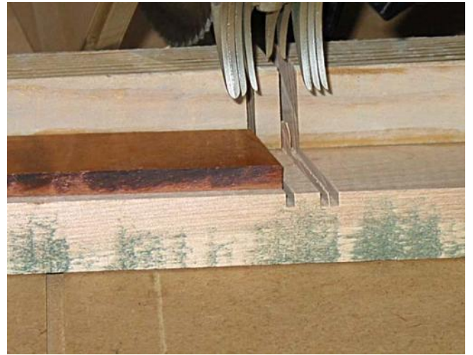
Close-up of the L sacrificial fence. Notice the saw kerf, which helps cut to correct length.
