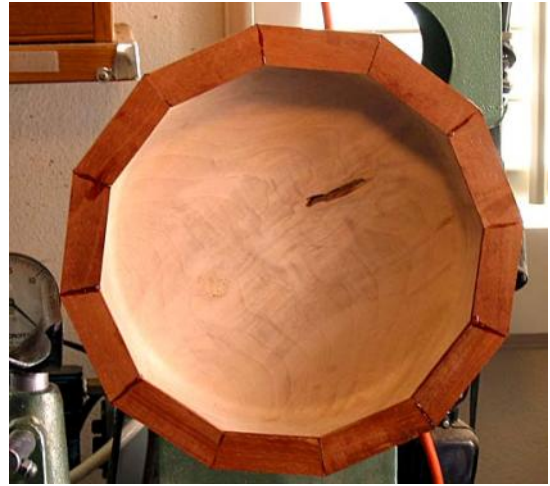
All segments glued in place. Next step is to turn rim to final thickness and shape.
