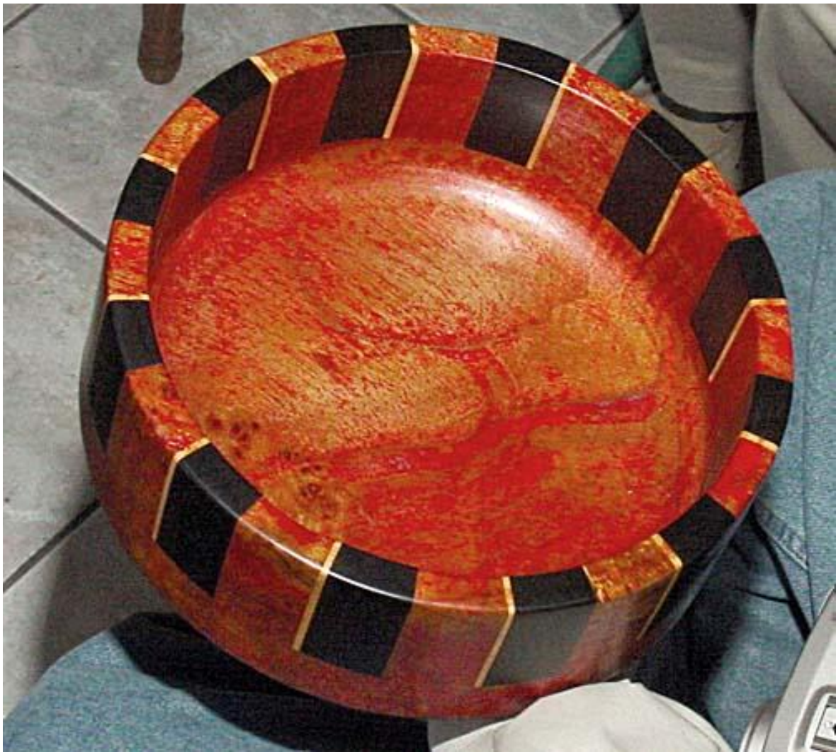
This photo show a bowl with the inlays placed into vertical cuts made with the chop saw.
