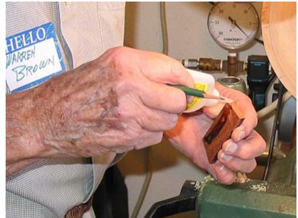
Applying CA glue between the pencil lines showing where segment contacts the rim.
