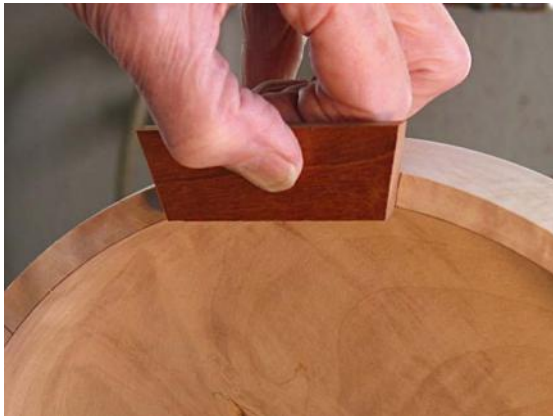
Positioning the first decorative segment for glue up.
