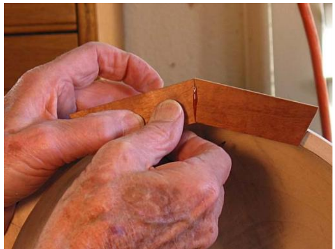
Gluing in the second segment.
