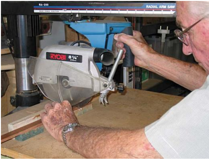
Warren uses a radial-arm saw to cut the segments
